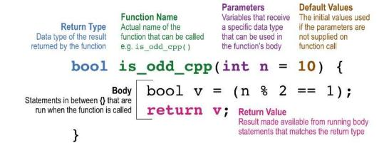
Fig. 1. Graphical annotation of the is\_odd\_cpp function.
